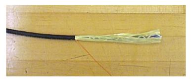
Figure 5 – Remove the 5" section of outer jacket.
