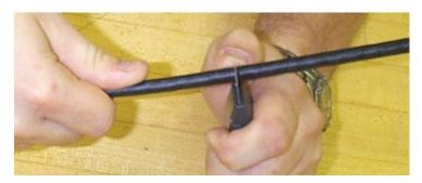
Figure 3 - Ring cut the cable.
