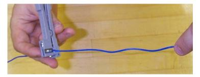
Figure 23 – Score the buffer tubes as required.
