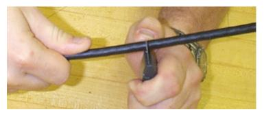
Figure 16 – Ring cut the cable.
