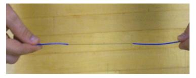
Figure 25 – Remove the buffer tube.
