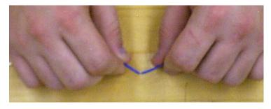
Figure 24 – Flex the tube at the score mark.
