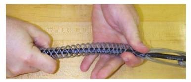
Figure 2 – Slide the grip about 20 inches beyond the cable end.
